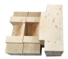
Hot blast furnace silica brick is a siliceous refractory brick with the main crystalline phase of tridymite. It is used to build the high temperature part of the hot blast furnace. Under the condition of long-term high temperature and load, the product volume is stable, high temperature creep is low, and can be used continuously for one or even two blast furnace ages.
